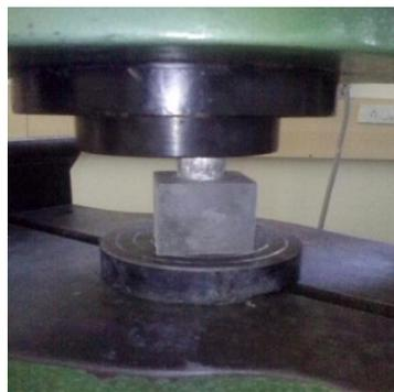
*Fig 4. Compression Test*
